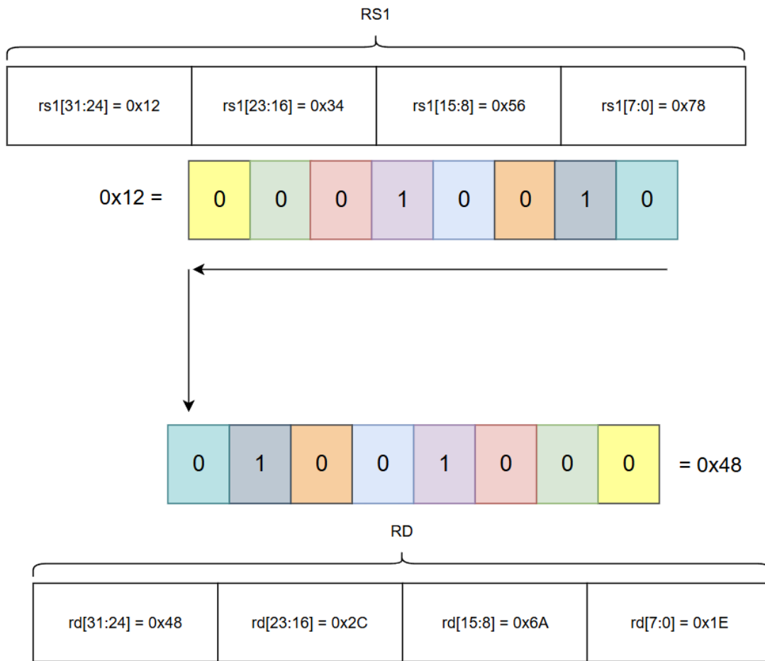
Figure 4.6: Execution of the brev8 instruction, demonstrating internal bit reversal per byte. Source: Author.
